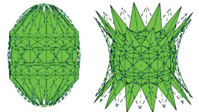
This illustration shows how one designed origami crease pattern would fit both a 3D elliptical surface (left) and a hyperbolic surface (right).
