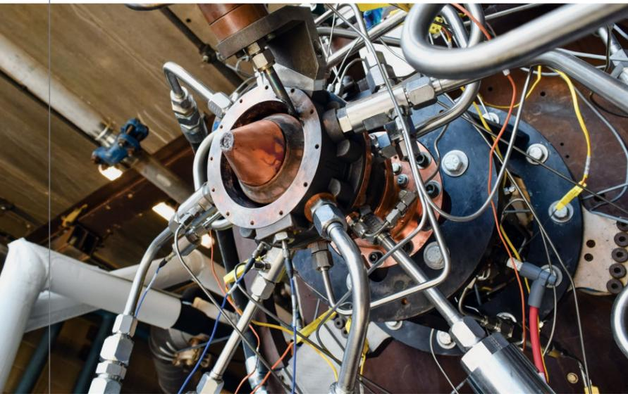
*In a rotating detonation engine, the combustion wave propagates continuously around the ring-shaped channel between the inner and outer sections. The liquid-cooled engine above, designed at Purdue and 3D-printed by NASA, still fires up even after enduring dozens of runs at Zucrow Labs.*
