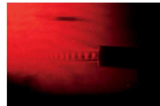
This demonstration of Schlieren videography shows diamond-shaped pressure gradients in the air exiting the nozzle of an aerosol duster spray can.
