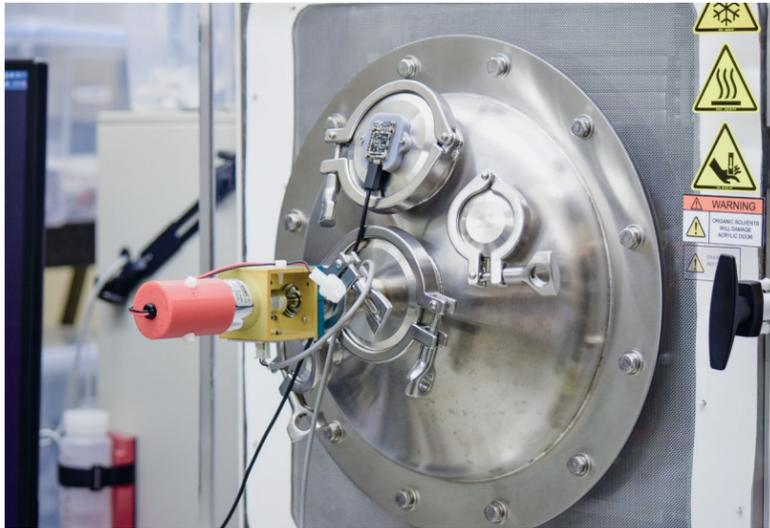
This device is a prototype of the microwave generator that LyoWave is preparing to bring to market. It is sized to fit on standard freeze-drying cabinet doors, which makes it easy for pharmaceutical companies to incorporate this technology into their existing manufacturing processes.
