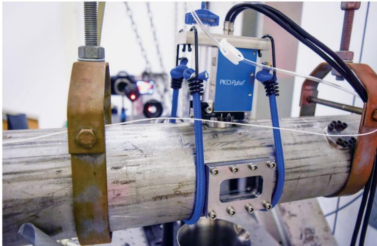
A test section of this shock tunnel has been fitted with a device that releases tiny water droplets in line with the viewing window. The water droplets will provide experimental results while also helping determine the appropriate timing for the shock wave when it comes time to test ice crystals.
