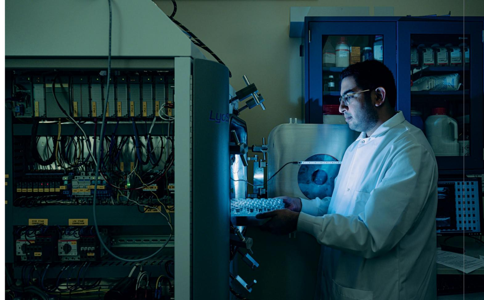
Ahmad Darwish, a senior research associate, removes a tray of vials from a freeze-drying cabinet that has been fitted with a microwave heating device developed at Purdue.
