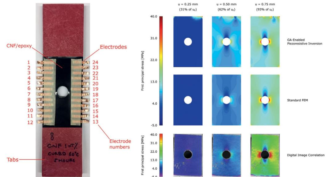
This electrical impedance tomography (EIT) experiment conducted by Tyler Tallman and Hashim Hassan shows conductivity change distributions in a specimen that is under tension. Tallman is finding the correlation between the conductivity change and the physical effects.
