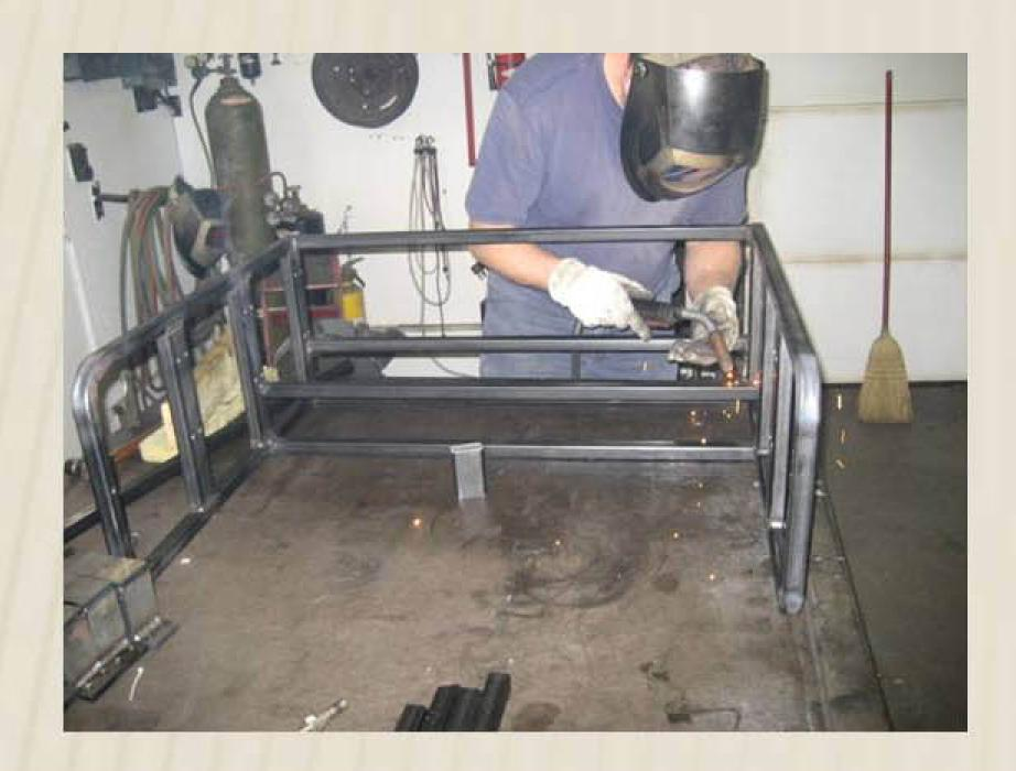
The spaceframe was designed to maintain the tight tolerances in shafts between the engine and transmission and to the driveshaft given the high deflection in the wood frame. In order to minimize the amount of steel needed, the space frame houses the engine and transmission as well as connects the rest of the vehicle together. Clamps hold the front and rear sections of the frame together and supports on the top and bottom keep the spaceframe from moving along the frame.
