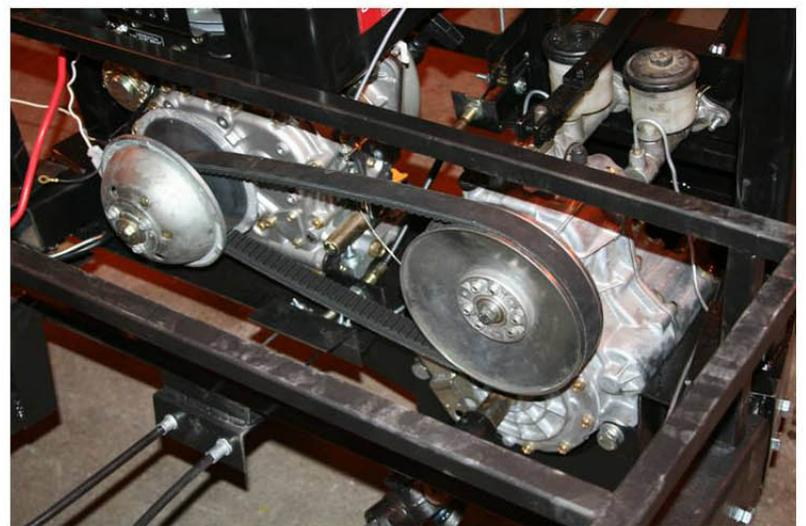
What we started with! (Left) Yanmar diesel engine, (Right) CVT Transmission coupled by belt
