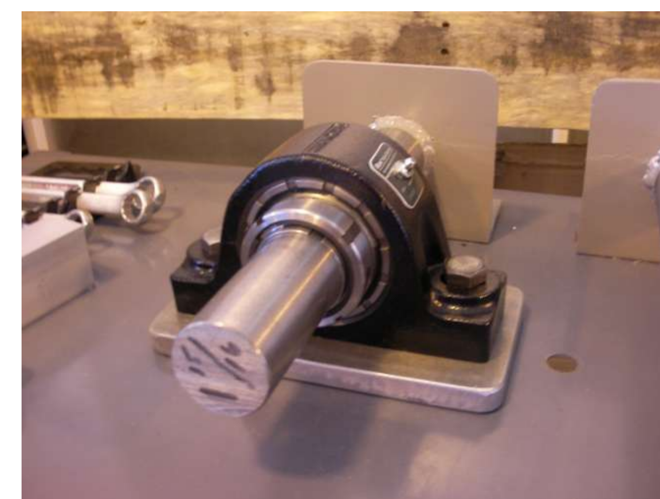
Rexnord bearing equipped with SHURLOCK technology.
