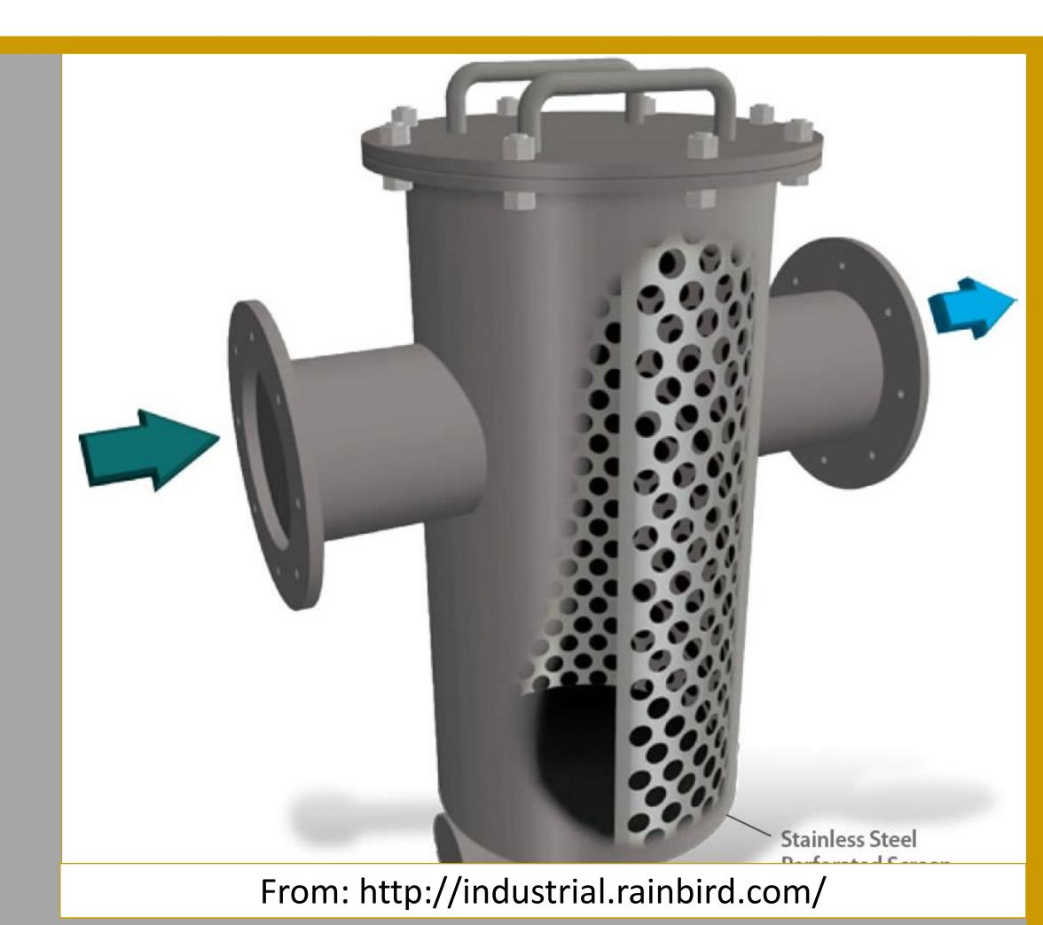
Screen Filter: Particle filtration method where screen catches particles and either blocks ones that are oversized or resizes them as they shear through the screen.
