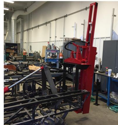
The post driver can operate at 1500 psi and deliver up to 3000 pounds of driving force. It is capable of driving up to ten foot sections of pipe forty feet into the ground. The weight of the driver is not an issue at a mere 500 pounds with the fact that the weight limit of the PUP is over 2000 pounds. It comes with stabilization legs and side to side tilt options for optimum performance.
