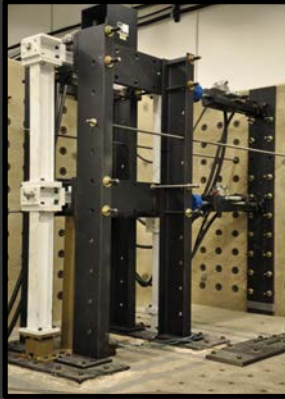
Modularized moment resisting frame specimen equipped with advanced vibration mitigation damping systems
