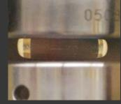
Unconfined 0.001/s strain rate Ductile response
