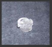
100 MPa confinement ~500/s strain rate Failed at PSD ~360 MPa
