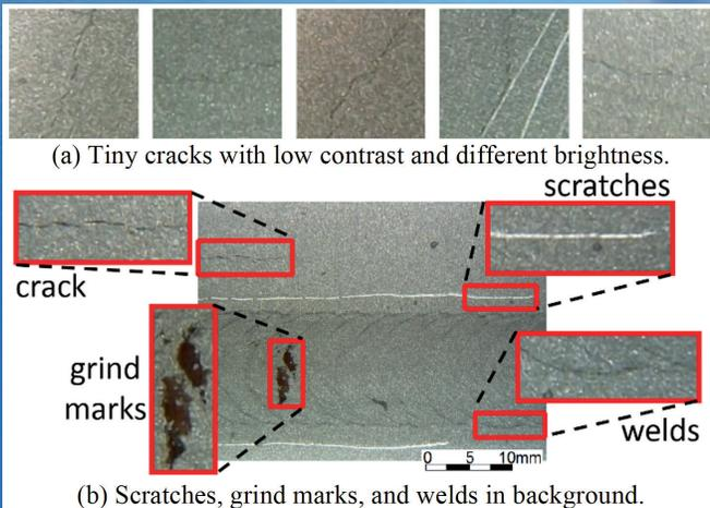
(a) Tiny cracks with low contrast and different brightness.
