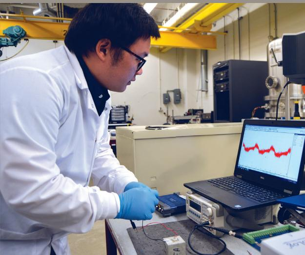
Civil Engineering PhD student Yen-Fang Su uses vibrations to test the strength of a concrete sample. The team plans to take its research into the field within a year.
