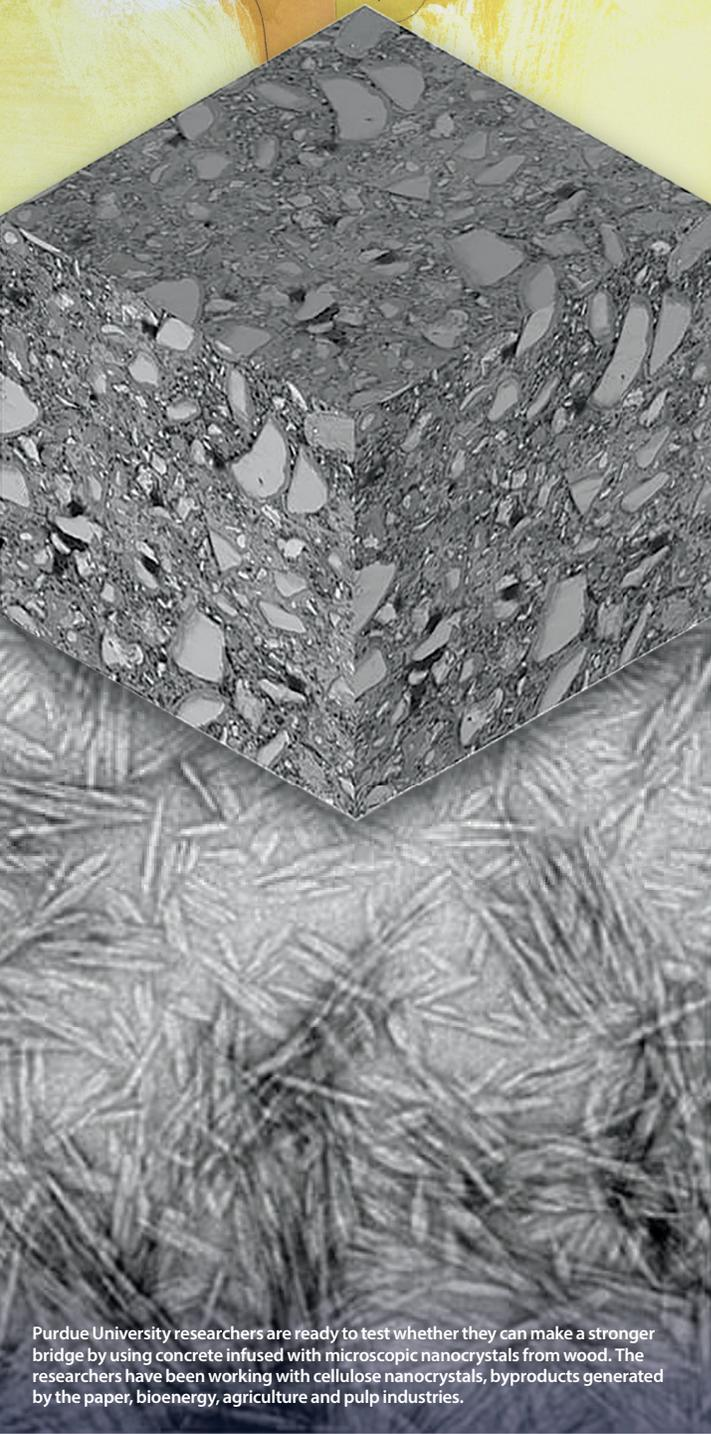
Purdue University researchers are ready to test whether they can make a stronger bridge by using concrete infused with microscopic nanocrystals from wood. The researchers have been working with cellulose nanocrystals, byproducts generated by the paper, bioenergy, agriculture and pulp industries.
